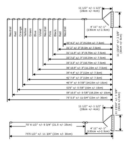
Note: For tournament-supplied handle sections, the bridle length shall be  $150 \text{ cm} \pm 2.5 \text{ cm}$  (4'11" 1") and the length of the handle shall be  $30 \text{ cm} \pm 6 \text{ cm}$  (11- 13/16"  $\pm$  2-3/8") (see diagram). For skier-supplied handles the tolerance on the bridle length is + 2.5 cm/-10 cm (+1"/-4").
